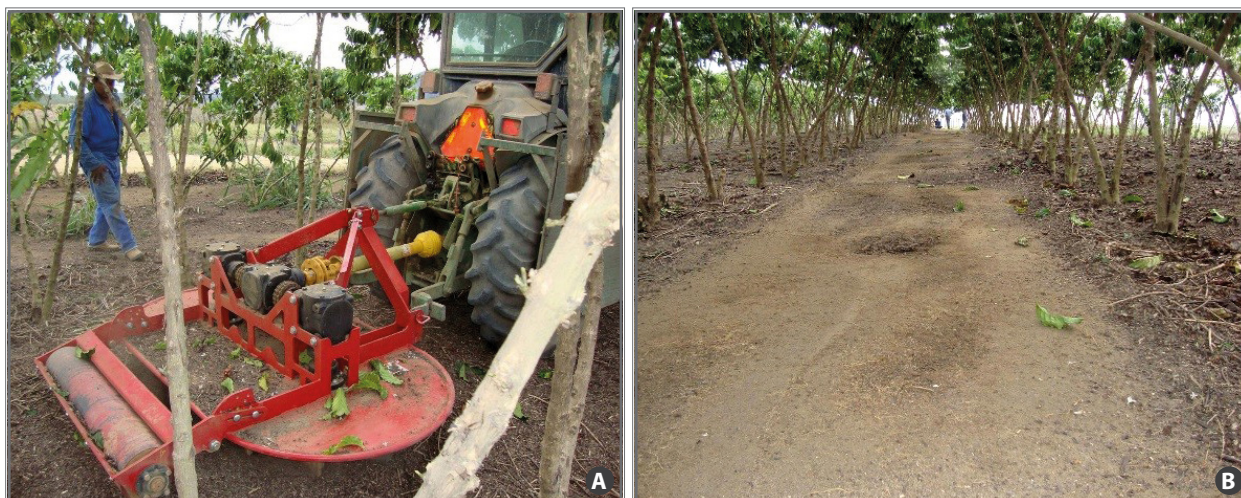
Figure 10. Planer coupled to the tractor used for leveling the ground before picking the strip harvested fruits on the ground (A); and terrain detail after the operation of the implement (B), in the 2012/13 harvest, in Nova Venécia/ES.
