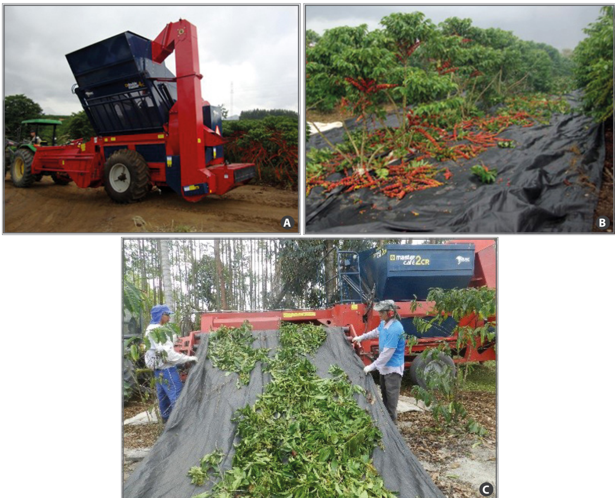
Figure 3. Machine adapted to collect leaves, branches and fruits (A) on the canvas (B) and detail of the canvas being rolled (C) in the 2014/15 harvest, in Jaguaré/ES.
