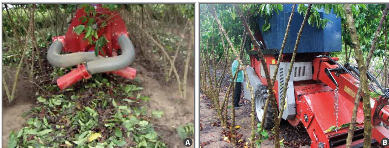
Figure 11. Traditional blower pulled by tractor used in the lining of the vegetal material before picking the strip harvested fruits on the ground (A); and ground picking process (B), in the 2012/13 harvest, in Nova Venécia/ES.
