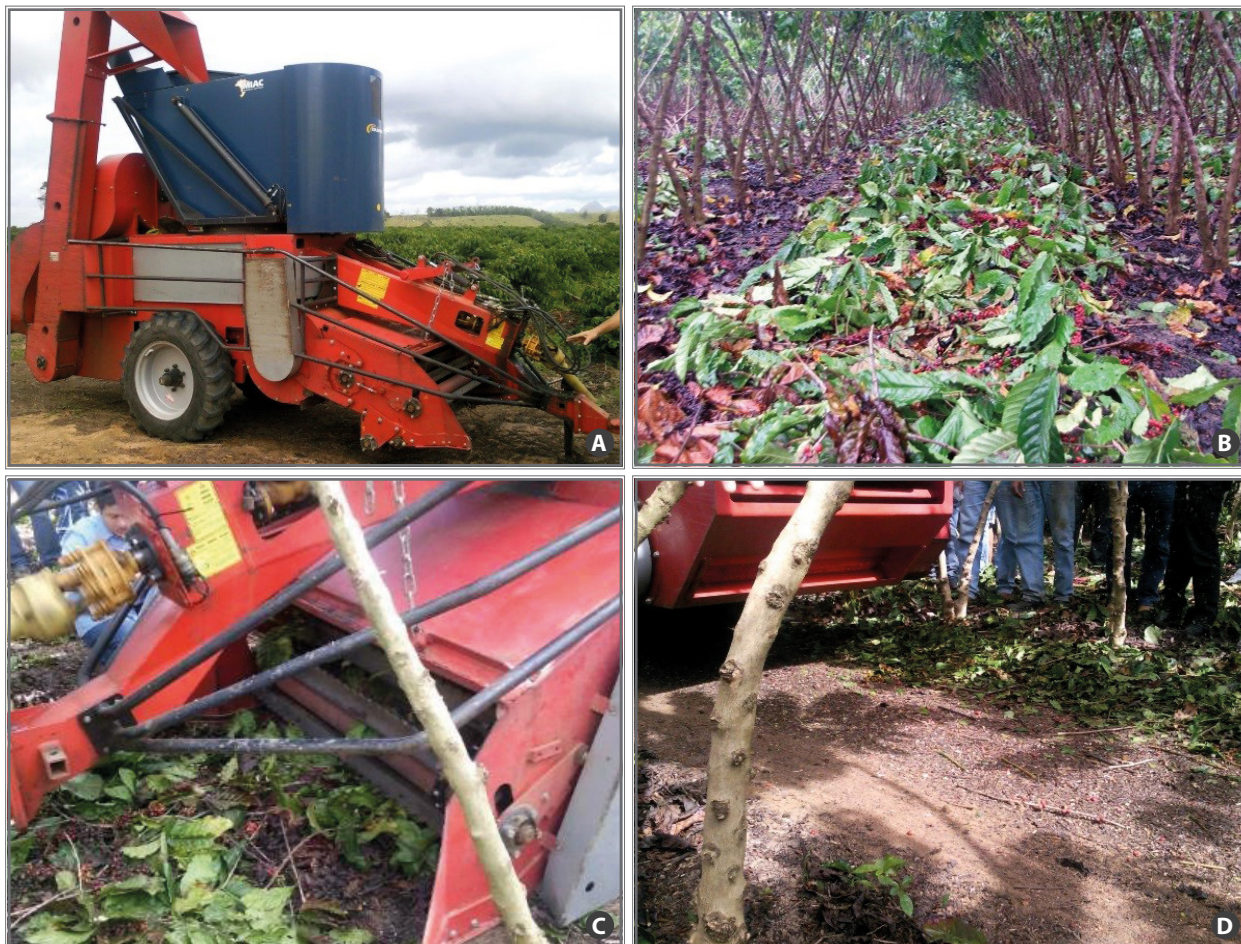
Figure 1. Machine used in the collection of conilon coffee fruits, strip harvested and left on the ground (A); detail of the strip harvesting associated with pruning (B); of the vegetal material collection operation (C); and image after the machine be used(D), in the harvest of 2012/13, in Nova Venécia/ES.
