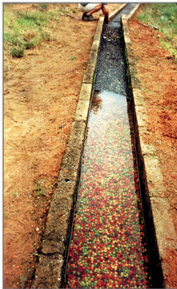
Figure 6. Washing and separation of green and ripe fruits from the dry ones, by density.
