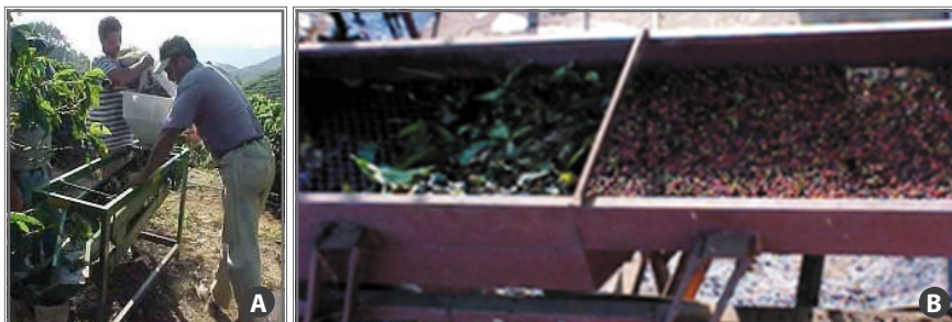
Figure 3. Mechanical separation of impurities in the field (A), and in the processing unit (B).
