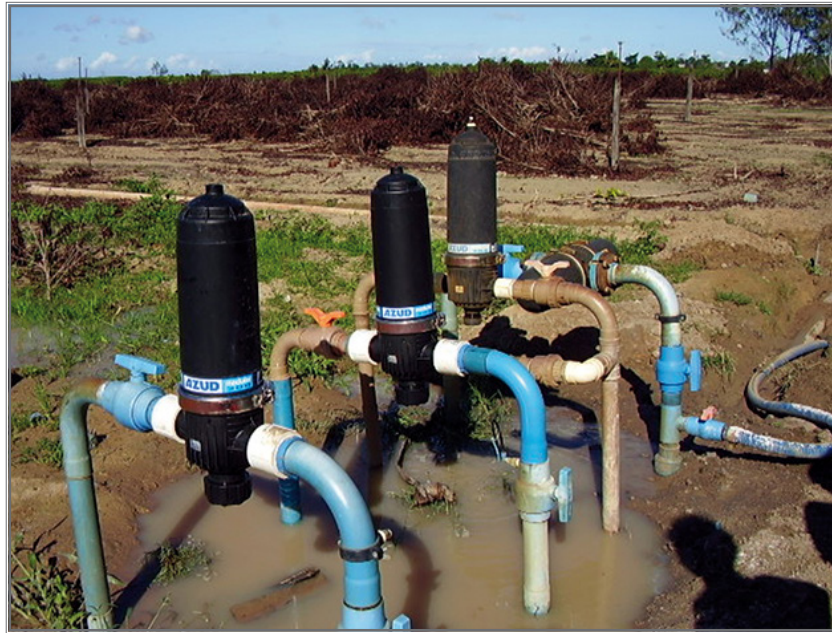
Figure 9. Control station components of a localized irrigation system.
