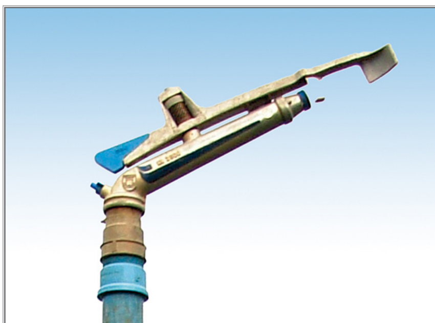
Figure 4. Hydraulic cannon used in coffee irrigation.
