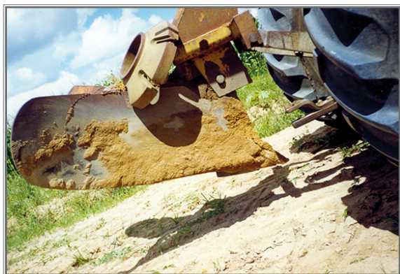
Figure 1. Furrower with variable depth and width, used in the crops implantation in flat relief soil.
