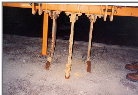
Figure 3. Three-point hitch subsoiler for breaking the compact soil layers and fertilizers mixing.
