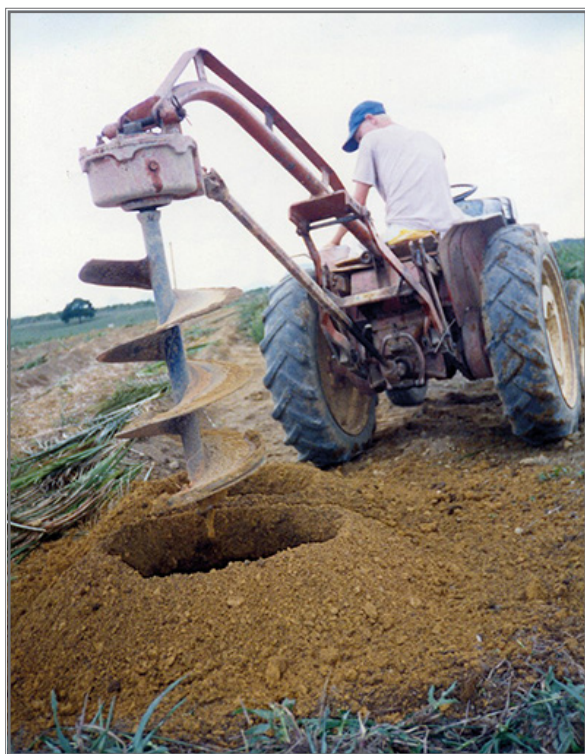
Figure 6. BDrill - soil drill of 18" diameter used in the opening of furrows.
