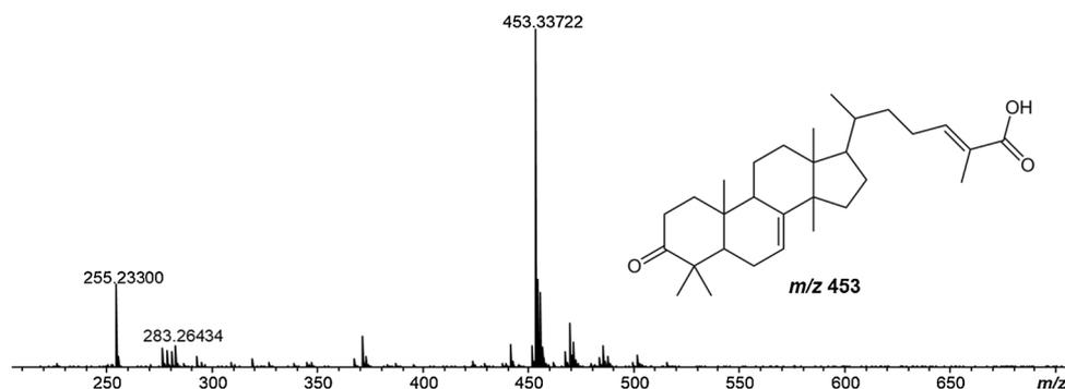
Fig. 3. ESI(-)-FT-ICR mass spectra of dichloromethane fraction of the residues.
