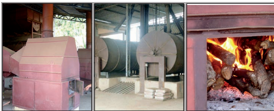
Figure 26. Drying in a mechanical dryer, with the use of an indirect fire.
